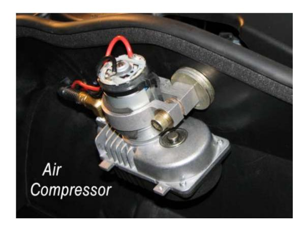
For a rider to easily go between one and two riders, with and without gear a simple, efficient and compact on-board air compressor was employed. And to control the air-compressor there needed to be a simple and effective switching method.
