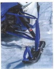
spot-on, as the sled tracked exactly where we wanted it, but in these trail conditions the system didn't separate itself much from other designs. At the first stop, Karpik tapped a bleeder valve on the air compressor to drop the rear air shock to 58 PSI, then we were back on the attack.
